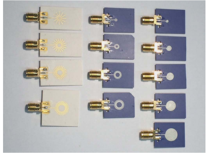
Fig. 5. Example of LTCC inductor prototypes. Left (first column): using Themex ceramics technology. Right (two next columns): using Heraeus technology.
